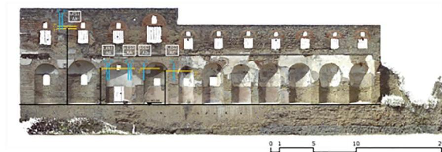
Scheme of GPR measurements on the Southern façade of the Sarno Baths building
