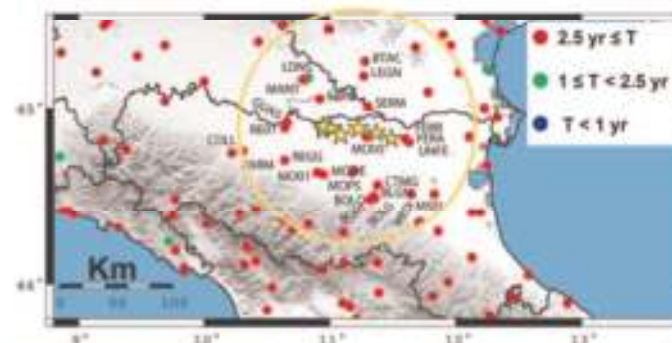
Figure 4. GPS stations lying within 100 km (yellow circle) from the May, 2012 Emilia earthquakes (yellow stars). The colour of circles indicates the observation time span ( T ) in years (inset).
